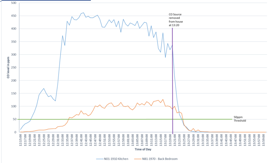
Figure 3.10. CO- Lascar data logger outputs for the highest readings in 1920 and 1970 houses
